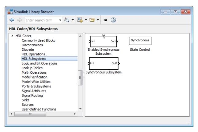
Use the State Control block with Simulink, DSP System Toolbox, Communications System Toolbox™, or Vision HDL Toolbox blocks that support HDL code generation.
