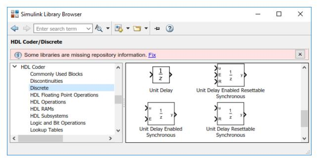
The blocks use the Enabled Delay, Resettable Delay, and the Enabled Resettable Delay block with a **Delay length** of 1 in combination with the State Control block in **Synchronous** mode. The synchronous behavior of the State Control block generates cleaner HDL code and uses fewer hardware resources.
