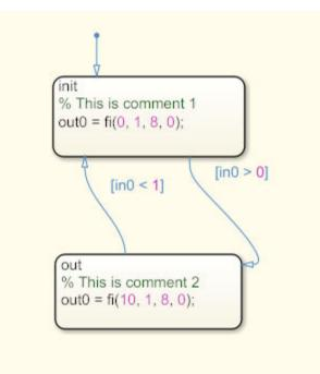
When you generate Verilog code from the model, HDL Coder displays the comments in the Stateflow Chart inline beside the corresponding Stateflow object.
